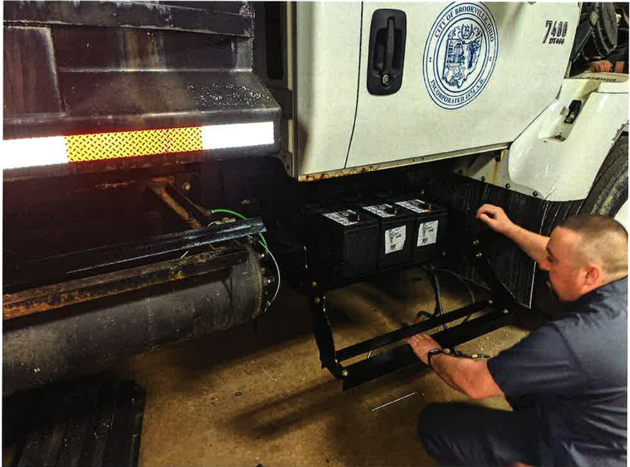
The Service Mechanic installs a new battery box and a step on one of the department's large dump trucks.
